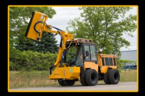
The Trackless Boom Flail Mower is perfect for those difficult, unsafe or impossible areas to mow. Ditches, steep inclines, over guard rails and waters-edge are areas in which the boom flail excels. Hydrostatic speed control allows the operator to react to oncoming obstacles for optimum safety and productivity.
