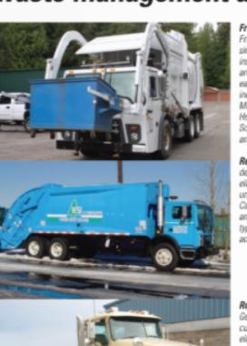
Front loaders - LoadMan Front Loader scales are a simple bolt-on system that installs in a few hours. They are designed to perfectly fit each truck's specifications including those built by McNeilus (Atlantic and Pacific), Heil, Wayne Engineering, Scranton Manufacturing, and Labrie.
