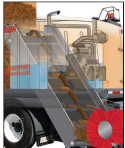
Elgin conveyors are designed to be interchangeable should a customer have different applications throughout the sweep season.
