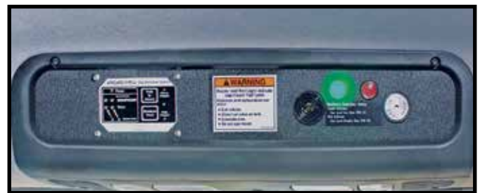
Optional In-Cab Mounted Methane Detection
