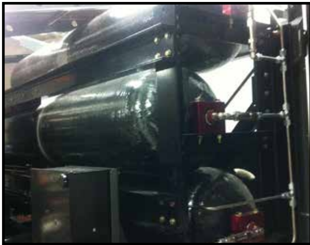
3600 PSI Composite Fuel Tanks
