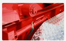
All trailer hoists have dual safety props to add extra security when the hoist is in the up position. 7 rollers per side help aid the container as it is loaded or unloaded on the hoist. Each roller is equipped with a bearing and a grease fitting for easy rolling and maintenance.
