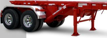
\*EX model shown with following options: aluminum diamond plate fenders, aluminum rims and premium red paint. Standard has black paint, quarter poly rear fenders and steel rims.
