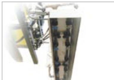
The construction of the spreading bar offers protection for pipes and nozzles and ensures accurate liquid spraying.
