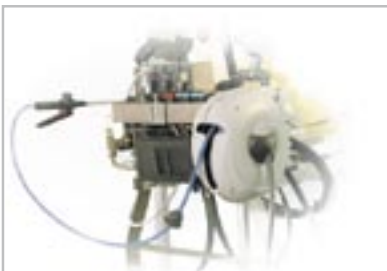
Hand-held lance sprayer and 12 m hose drum for hard-to-reach places, such as stairs or shop entrances etc.
